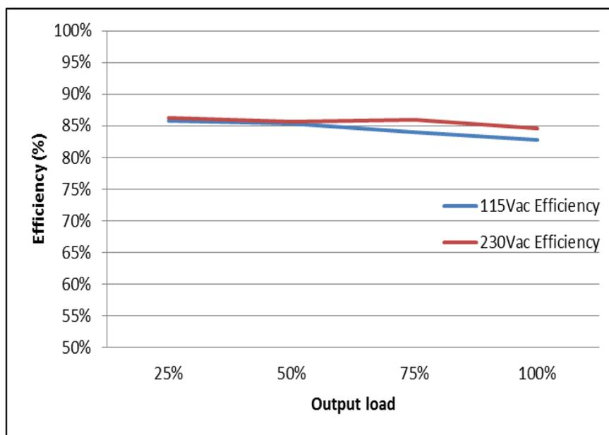
Fig.1 Efficiency versus output load
